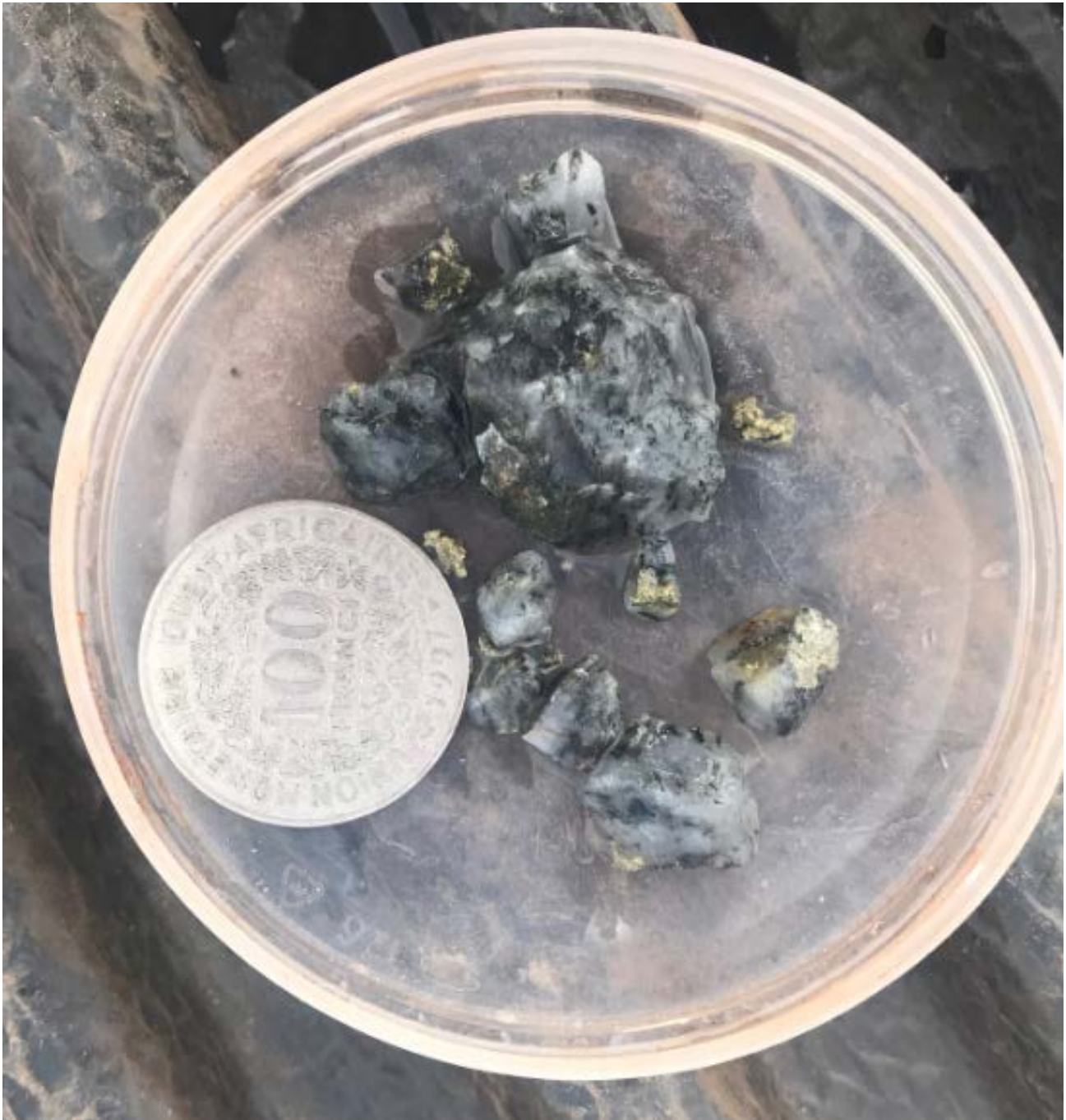
Figure 10: Gold panned from RC drill hole 19FARC008. A 1kg sample (56-57 metre interval) was panned and yielded a number of coarse gold fragments. This interval assayed 102.38g/t Gold. Scale diameter coin 26mm.
