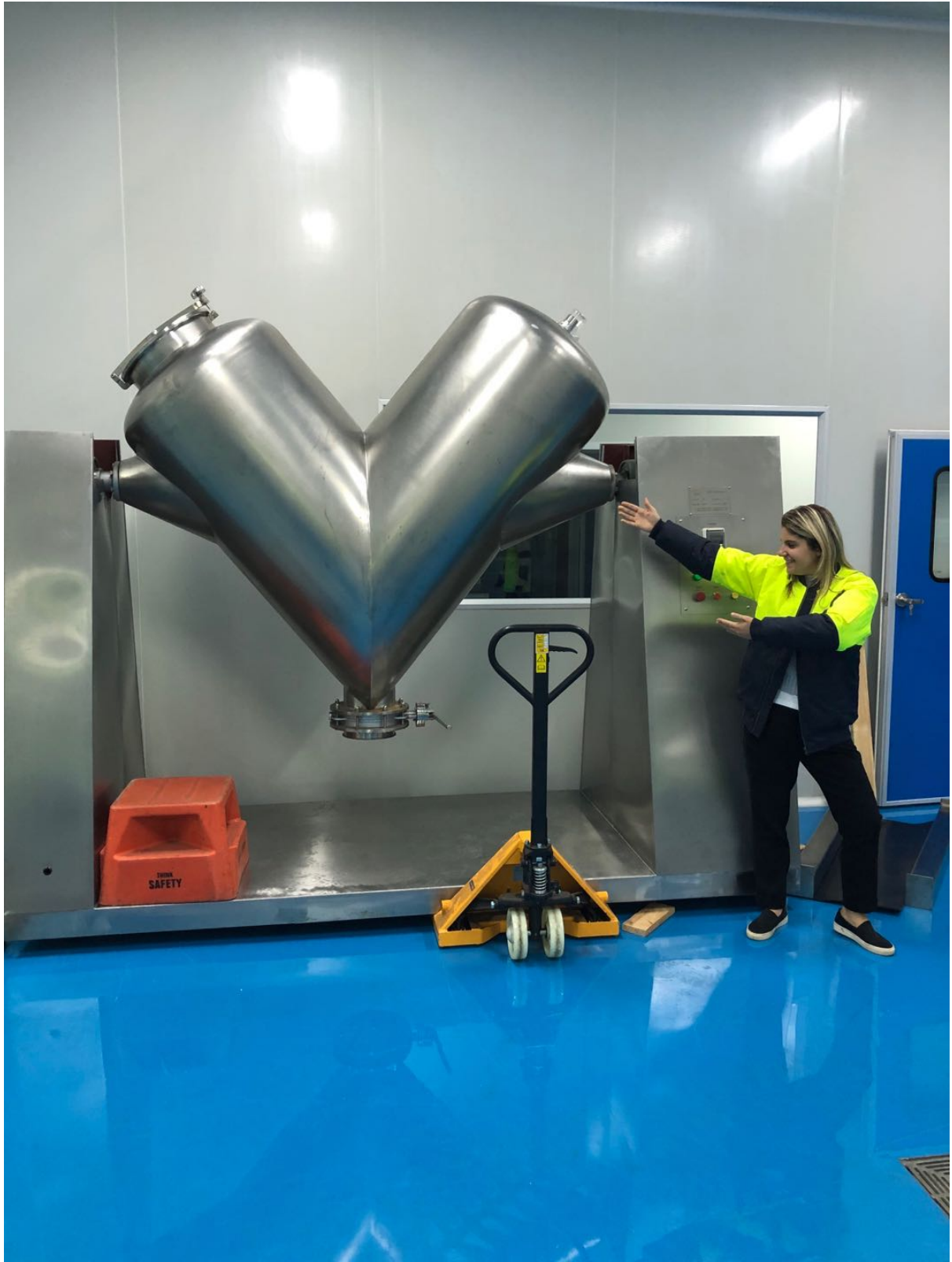
Above: New powder blender at FOD's Mill Park facility in Melbourne
