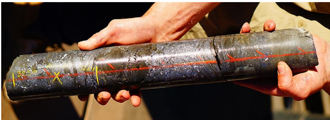
Image: Semi massive galena replacement. ACD080, 32.8m. Part of an interval 25.7m to 37.9m (12.2m) of well mineralised core consisting of strong galena (metallic grey), some pyrite and minor sphalerite.
