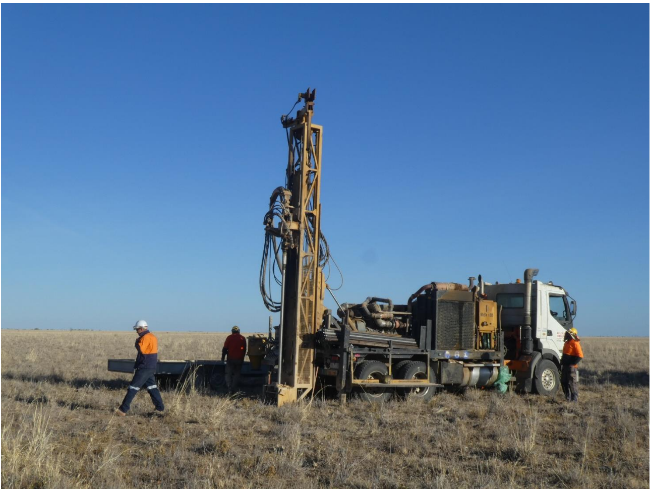
Figure 10: Infill drilling at the Lilyvale Vanadium project
