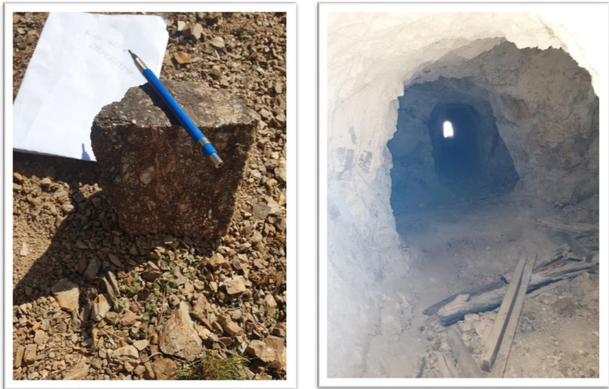
Figure 2: Left; Rhyolite breccia taken from the Specimen Hill Mine. Right; View from inside the Specimen Hill Mine; the walls are sulphide rich brecciated rhyolite and gold bearing quartz veins.
