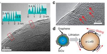
Samsung, Nature Communications 8:1561. Graphene balls for lithium rechargeable batteries with fast charging and high volumetric energy densities.
