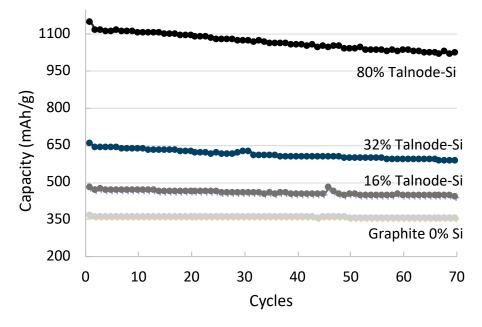
Talga graphene-enhanced silicon anode blended into commercial graphite anode
