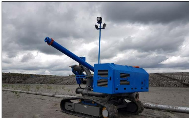
Figure 5\*: Water cannon typically used for hydraulic mining
