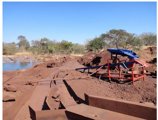
Sluice boxes and ponds
