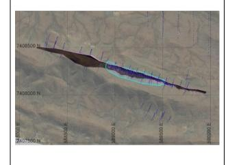
Long Section View - 7408250N looking north — Peake with drillhole traces and mineralised domains. Grade contol holes shown, but not used for estimation. Current Peake pit extents shown in light blue.
