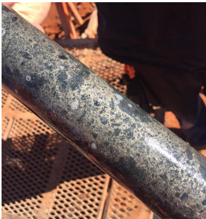
Figure 1. Breccia textured sulphide (pyrrhotite–pyrite–chalcopyrite) at 195m
