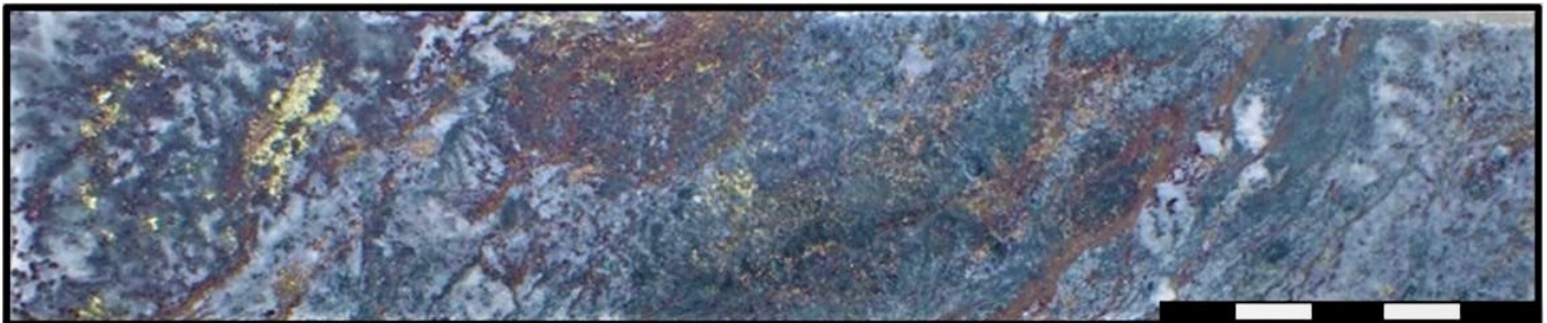
Picture 2: Drill core from KIODD002 (92.7m) – blebs of pyrrhotite-sphalerite-chalcopyrite hosted in quartz-chlorite-actinolite altered volcanic siltstone
