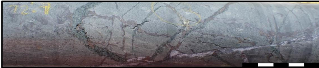
Figure 5B. Drillcore from KIODD002 (72.7m) – Pyrrhotite stringers with specks of chalcopyrite and actinolite – chlorite veins cutting chlorite – epidote altered volcanic unit.
