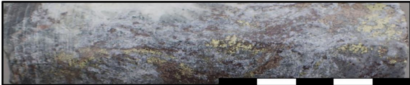
Figure 5D. Drillcore from KIODD004 (126.9m) – blebs of sphalerite – chalcopyrite – pyrrhotite in quartz – carbonate zone.
