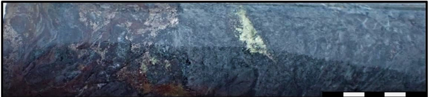
Picture 2: Drill core from KIODD002 (92.7m) – blebs of pyrrhotite-sphalerite-chalcopyrite hosted in quartz-chlorite-actinolite altered volcanic siltstone
