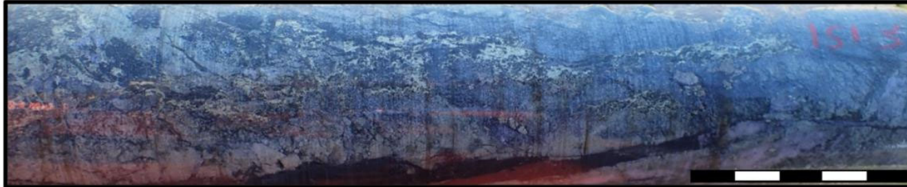
Figure 5C. Drillcore from KIODD003 (151.5m) – chalcopyrite ± pyrite blebs/stringers in chlorite – epidote altered volcanic unit.
