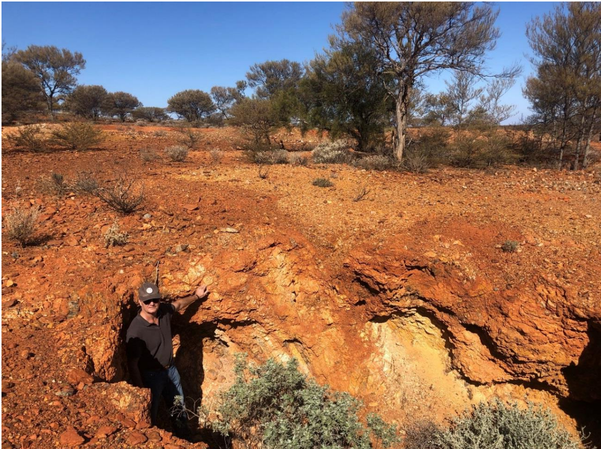
Image 2: Northernmost working at same location, confirming 330° strike and 60° dip to west
