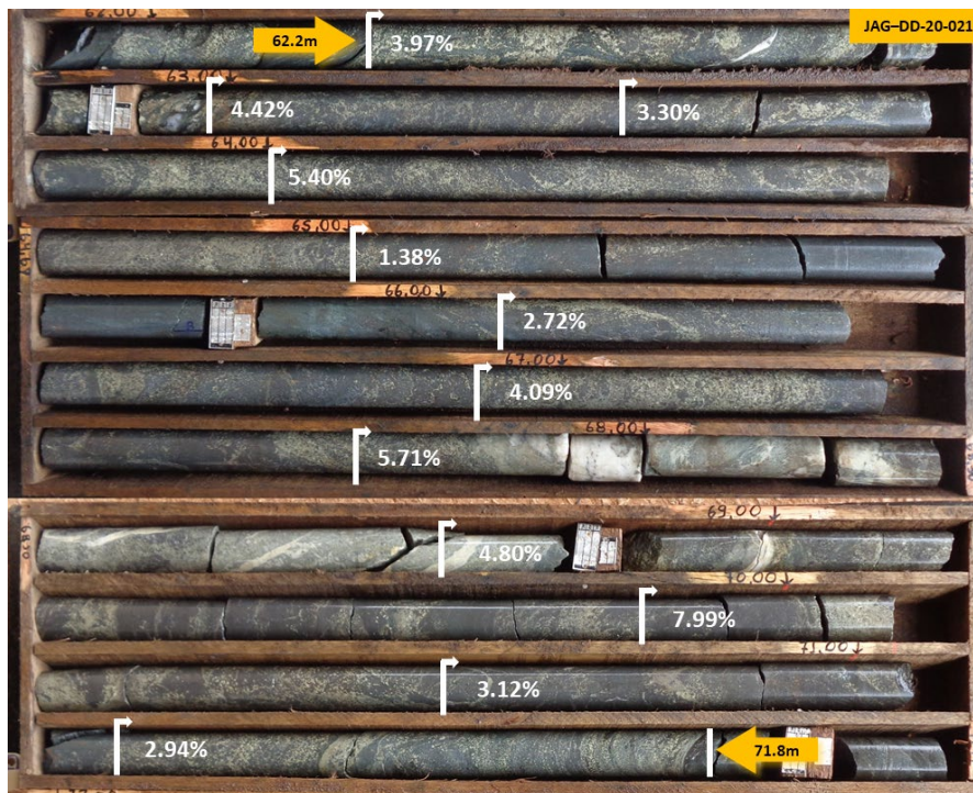
Figure 13 – Core photos from drill hole JAG-DD-20-021 at Onça Preta; 62.2 to 71.8m: This interval returned 9.6m at 4.19% Ni, 0.29% Cu and 0.16% Co.
