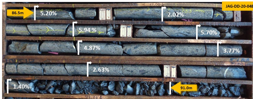
Figure 11 – Core photos from JAG-DD-20-048; 86.5 to 91.0m. This interval returned 4.5m at 3.66% Ni, 0.63% Cu and 0.17% Co.
