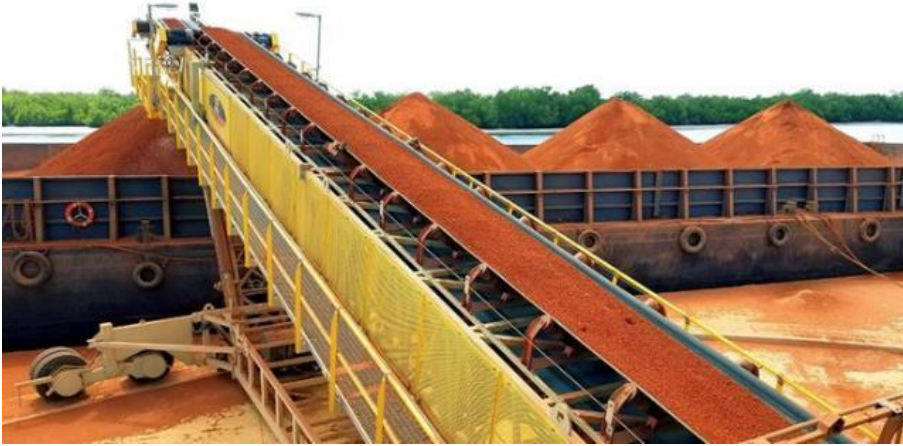
Figure 16 - Example of telestacker loading barges with bauxite.
