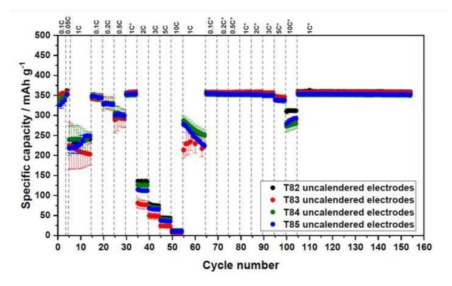
Rate capability tests were undertaken to analyse a range of different charge (C-rate) conditions.
