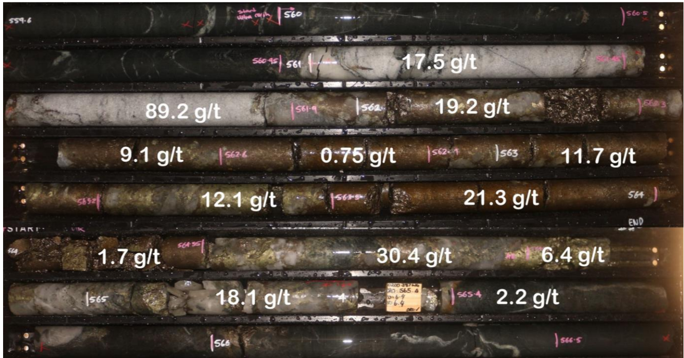
Figure 5: New drill core from the Viago Lode – hole DRDD387W4, high-grade shoot 40% milky and smokey quartz veins with semi massive pyrrhotite, trace chalcopyrite and abundant visible gold mineralisation. Interval assayed 6.1m @ 17.7g/t gold from 560.9m.
