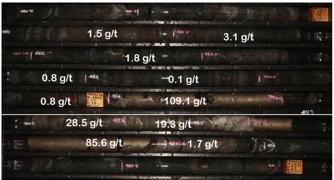
Figure 6: New drill core from the Deacon Lode – hole DRDD453A, high-grade shoot 20% milky and smokey quartz veins with semi massive pyrrhotite, trace chalcopyrite and minor visible gold mineralisation. Interval assayed 5m @ 23.5g/t gold from 481m.
