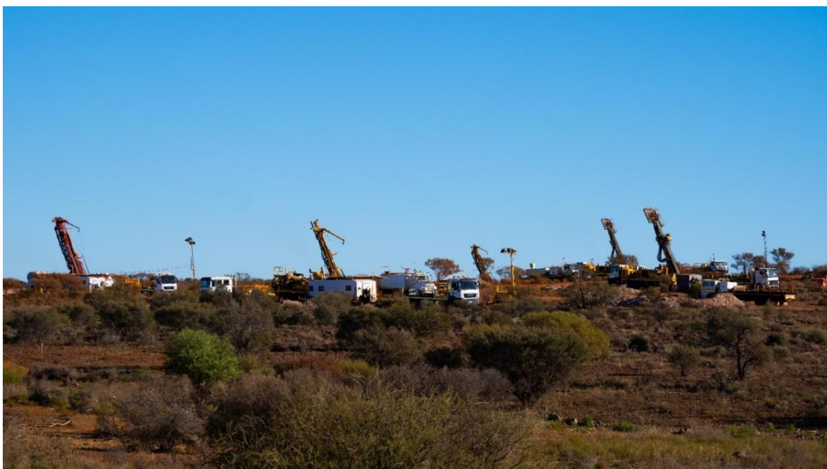
Figure 3: Diamond Drill rigs completing Resource conversion drilling at the Deacon Main lode at the Bellevue Gold Project. Further results are expected from ongoing drilling in coming weeks.
