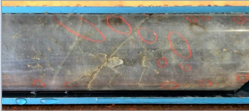
Typical silica-albite-sulphide Tura Lode mineralisation in BBRD1135 at 246.70m (assaying 184.63g/t Au); Multiple clusters of visible gold are circled*
