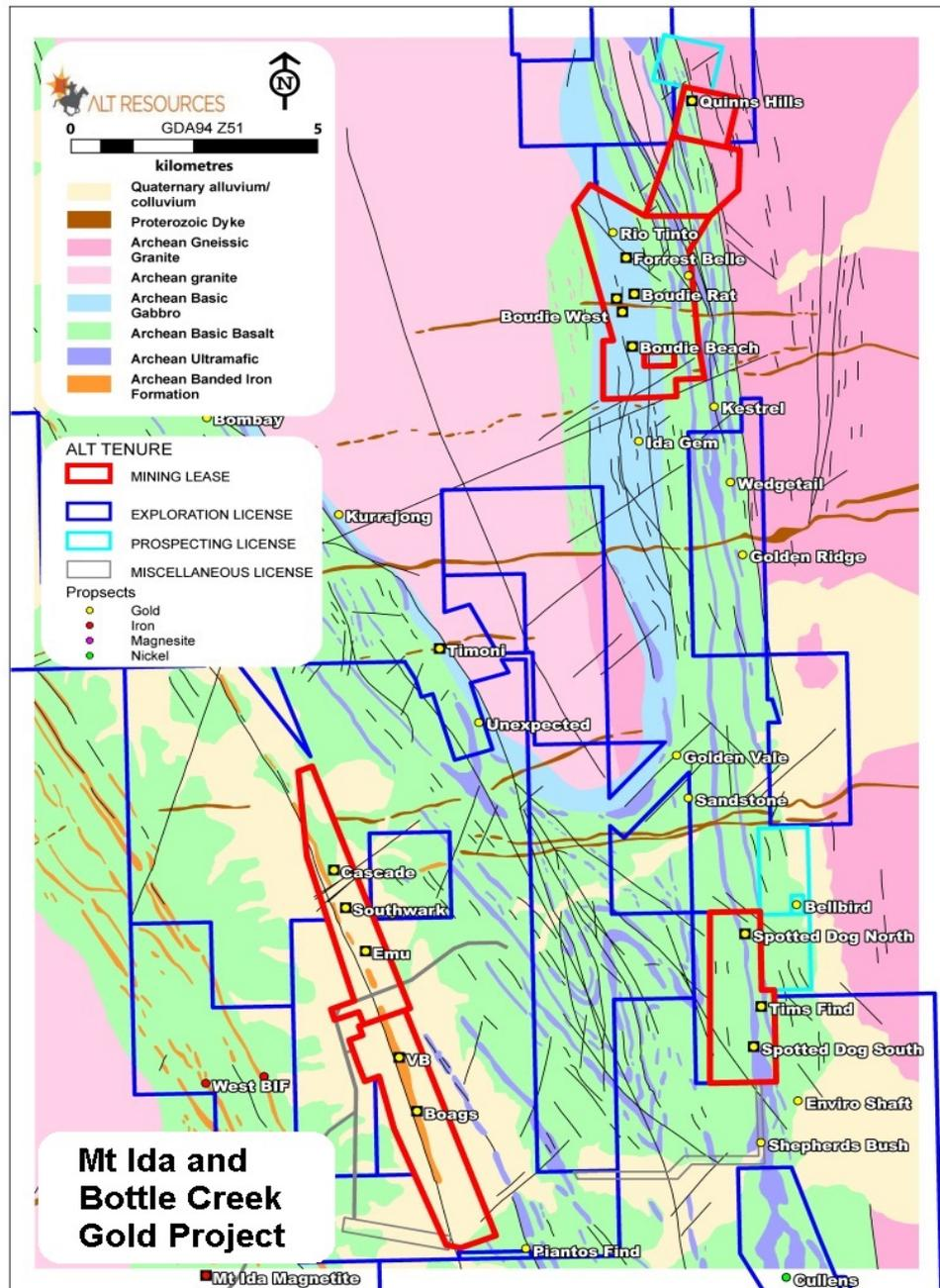
Figure 2: Geology of the Mt Ida and Bottle Creek Gold Project, Deposits and Mining Leases
