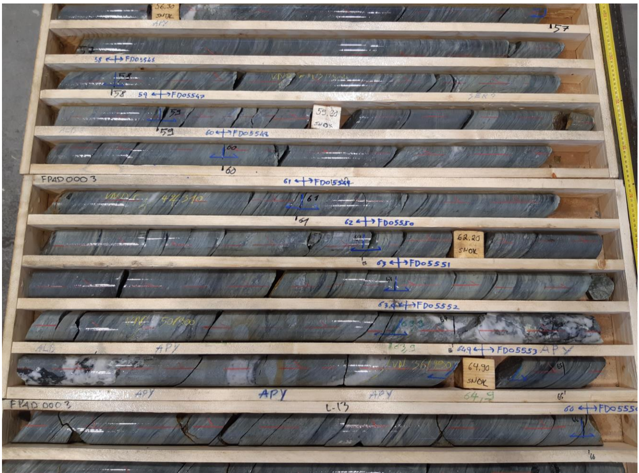
Figure 3: Diamond core from the first hole drilled beneath the Aarni' East base of till (BOT) gold anomaly, confirming the presence of intensely sheared and hydrothermally altered bedrock.
