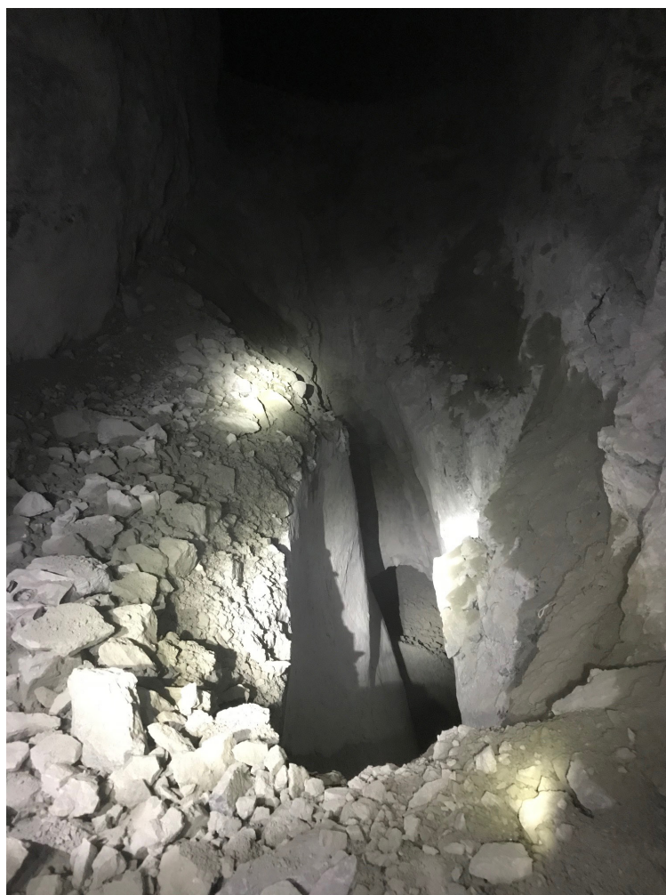
Avoca stope prior to backfill being placed
