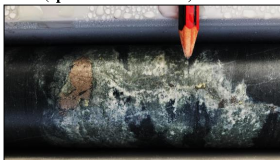
Clast of pyrrhotite , veinlet with ?chalcopyrite (62.0m)
