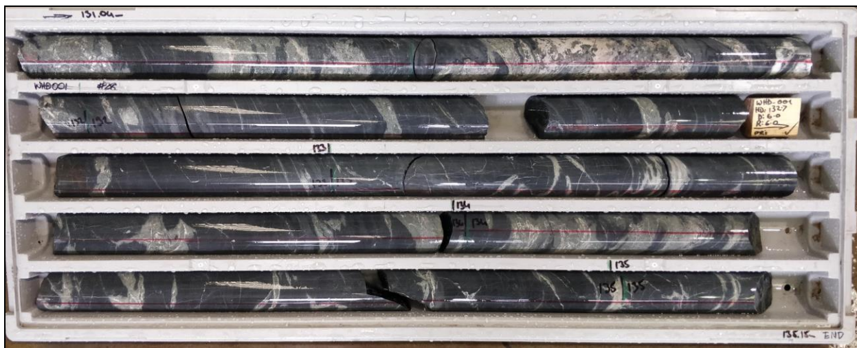
Core from 20WHD001 , 131-135.15m (sphalerite at 131.6m)
