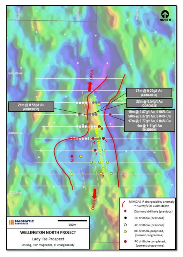
Figure 1: Lady Ilse Target, historic and current drilling locations, RTP magnetic imagery, IP chargeability summary
