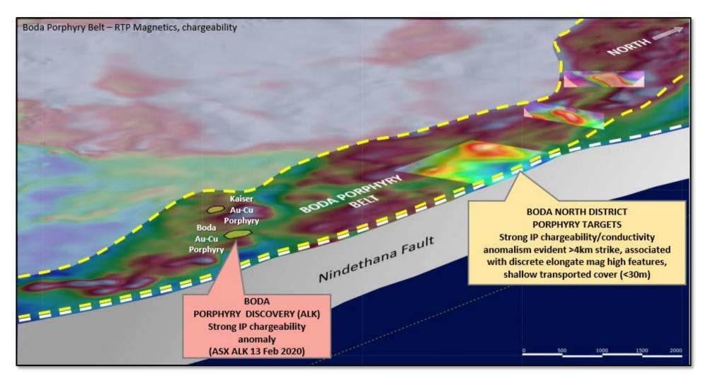
Figure 2: Oblique view of Boda Porphyry Belt, highlighting Boda North targets, characterised by strong chargeability anomalism, showing recent IP survey chargeability depth slice (ASX MAG 1
