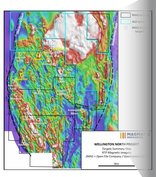
**Figure 3:** Aeromagnetic imagery, RTP (Magmatic and Open File Company/Government) showing northern Molong Belt porphyry target portfolio, Wellington North Project, highlighting Boda Au-Cu Porphyry Discovery (ALK), extensions to the Boda Porphyry Belt and target zones at Boda North, Boda South
