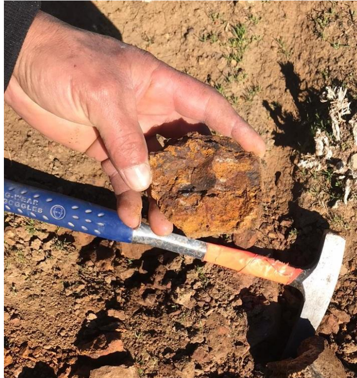
Figure 3: Colina2 Surface sample showing goethite-limonite alteration
