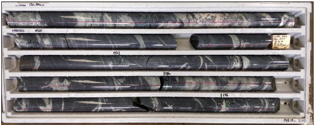
Core from 20WHD001, 131-135.15m (sphalerite at 131.6m)
