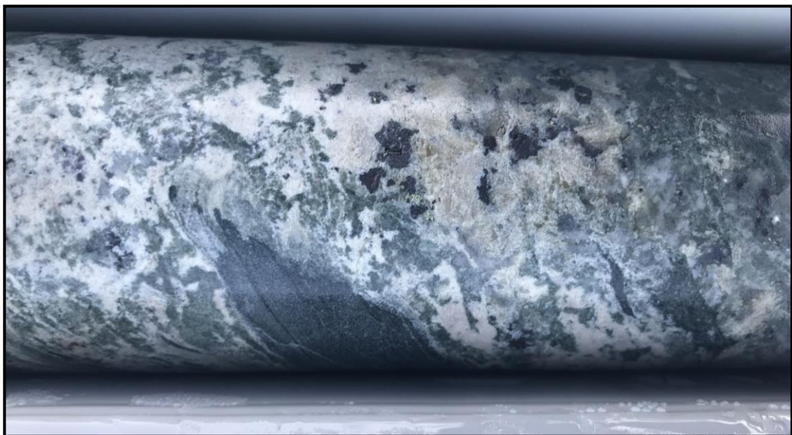
Fig. 4. Dark grains of sphalerite disseminated in an alteration band at 131.6-131.8.
