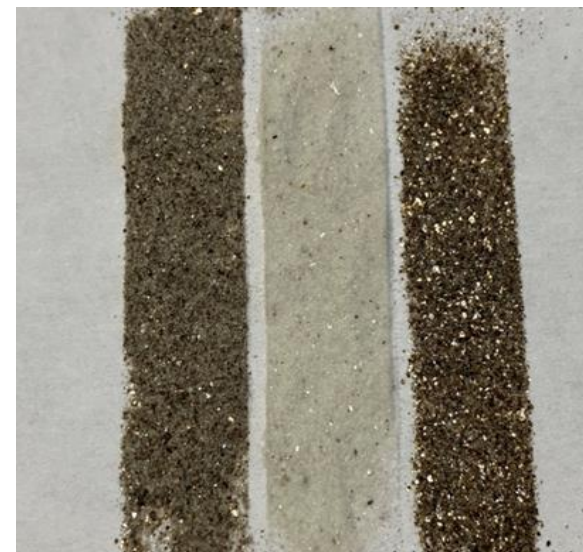
Gold plant leach residue (left), non magnetic reject (centre) and mica rich magnetic concentrate (right)
