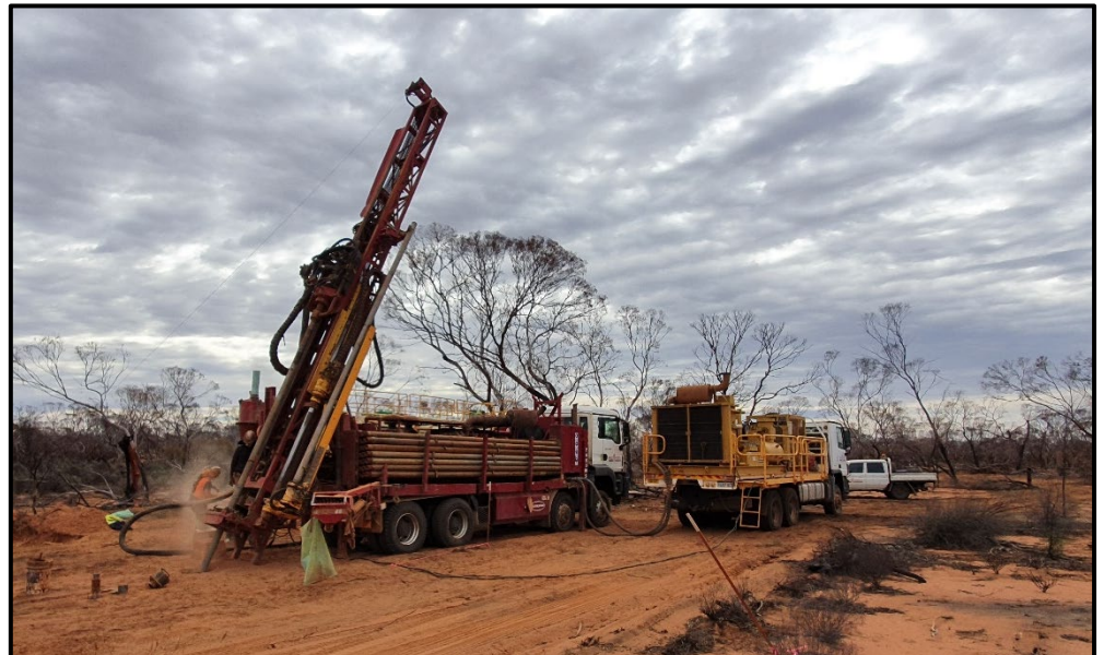
Figure 1 – RC Drilling at Galileo’s Lantern nickel prospect in the Fraser Range
