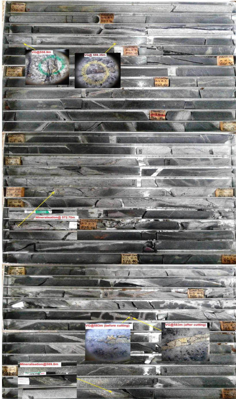
(Figure 1: Core boxes from TUDDH500 displaying high-grade mineralization discussed in this news release. Photos show a complex network of quartz-adularia veins. Host rock is monzonite. Quartz-adularia flooding extends for up to several cm beyond the veins. Open space vugs are also present. Gold, bright yellow, as well as pyrite, brassy yellow, and galena and sphalerite, grey, are present. Hole TUDDH500 is currently at a depth of 641.4m en route to its targeted depth of 1,000 m. This hole is designed to undercut the entirety of the main Tuvatu lode system in an area where a root feeder is hypothesized to be located.)
