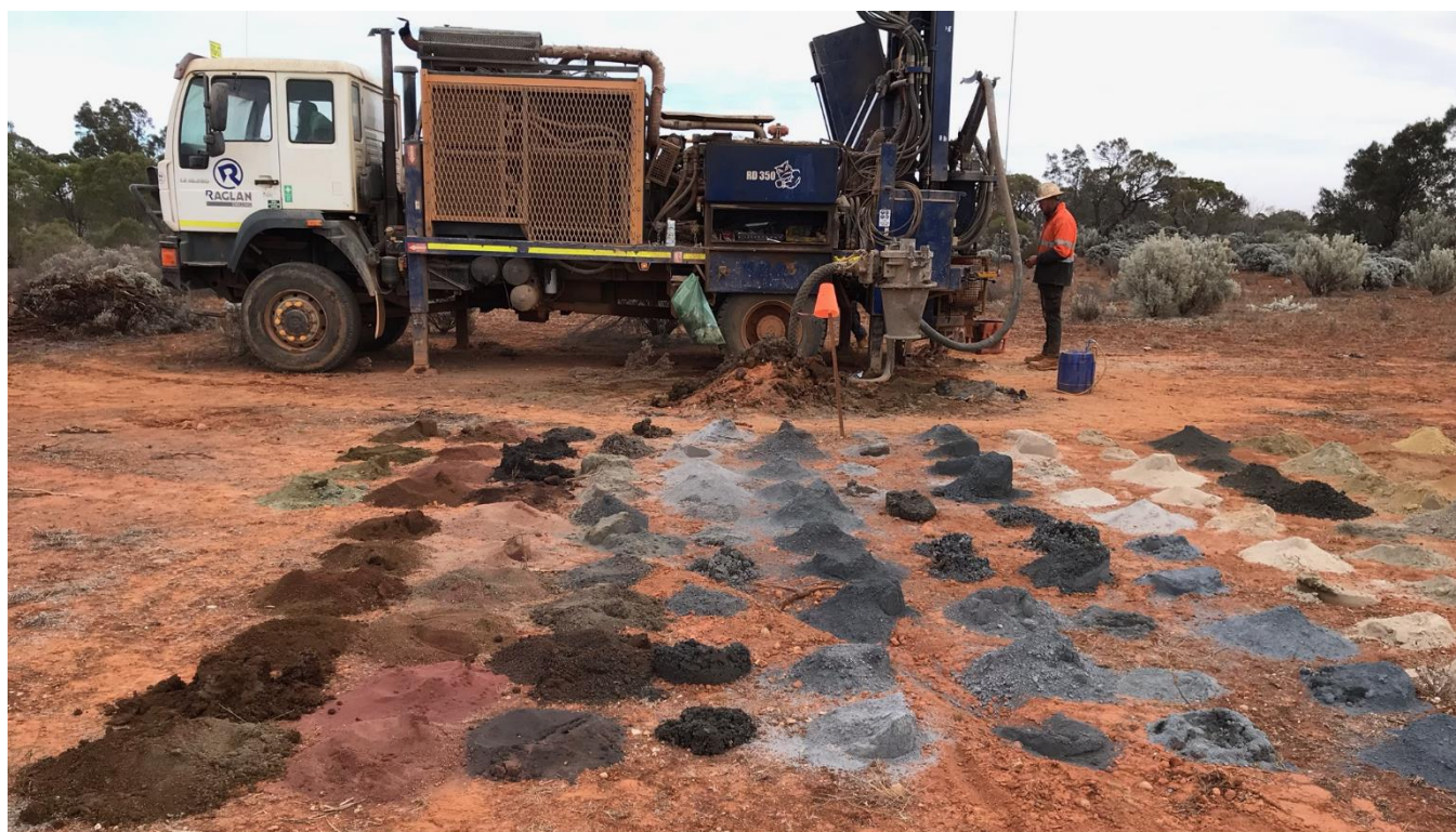
Figure 4: Air-core drill samples in the Fraser Range.
