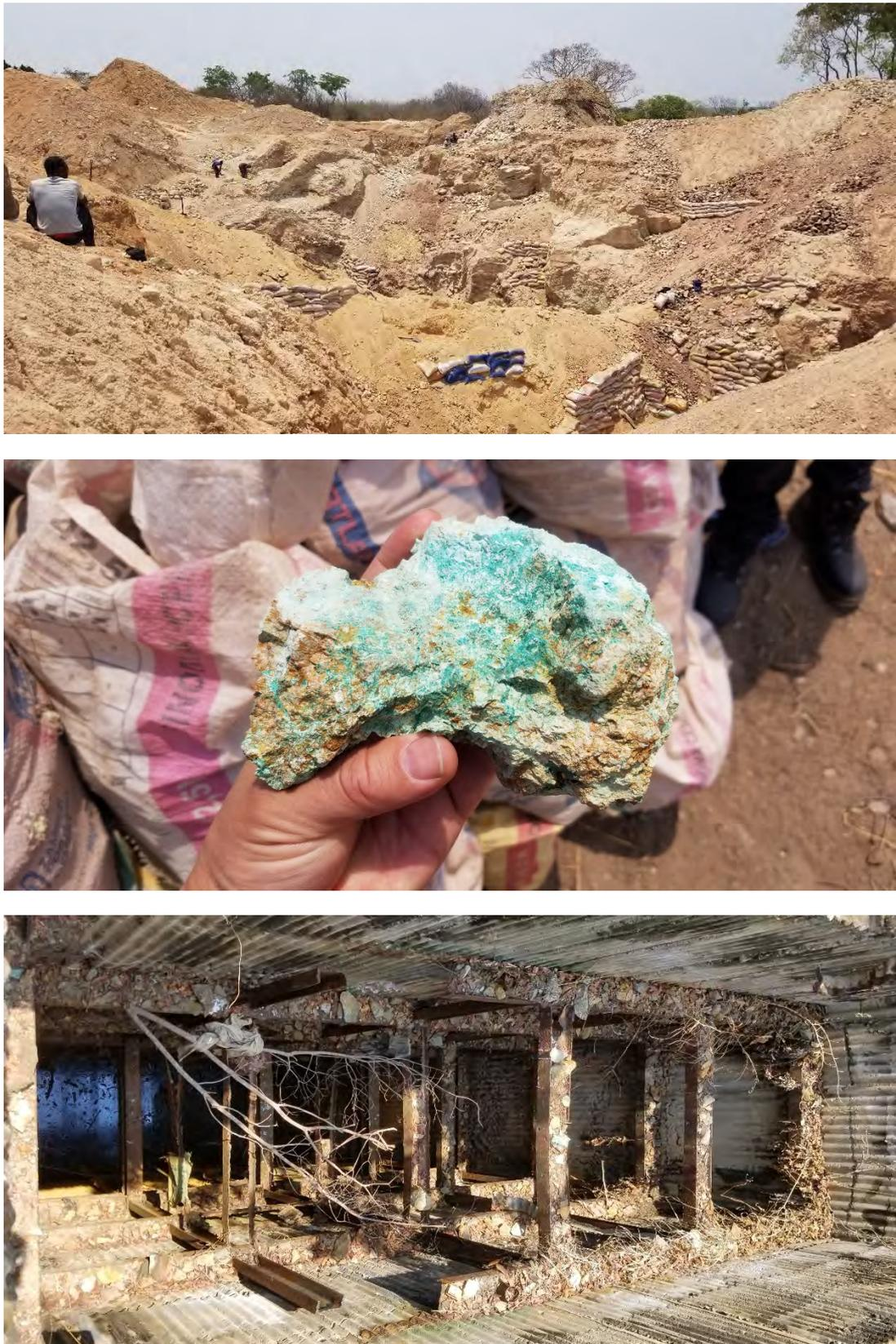
**Figure 6-19** Photographs depicting; the artisanal copper mining activity at the old 'Italian Mine' on the Mtuga Line (top); an example of the copper ore being packaged for sale to the Chinese (middle); and the Italian Mine flooded main shaft (bottom). Location centred approximately  $29^{\circ} 06' 52.3''\text{E} / 13^{\circ} 58' 19.7''\text{S}$  (Source: SRK ES, 2019)
