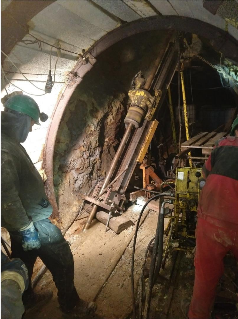
Image 1: Underground drill rig in operation at Sturec within the Andrej Adit
