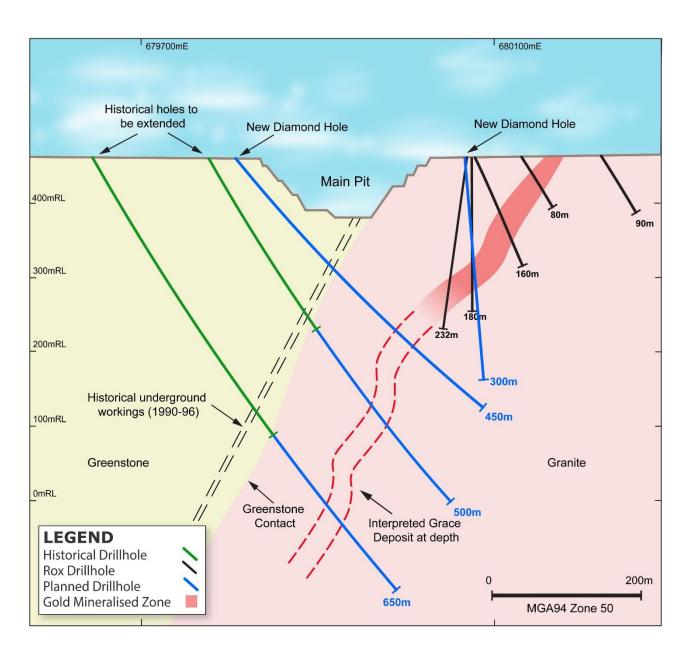
Figure 4 – Youanmi Main Pit and Grace Prospect schematic cross section showing planned diamond drill holes
