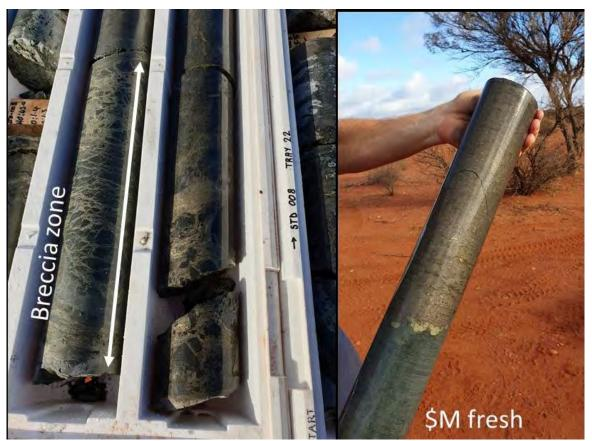
Figure 4 – photographs of drill core from STD008, one of the metallurgical holes completed at Stricklands. STD008 intersected 14.05m of nickel-copper sulphides from 36.7m downhole. The mineralised interval included massive sulphides (90-100% sulphides) between 36.7m to 46m (photo on right) and brecciated textured sulphides (50-75% sulphides) from 46m to 50.75m (photo on left).
