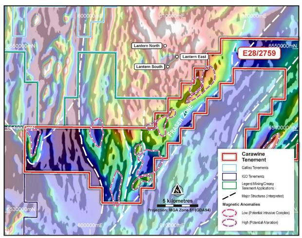
Figure 11: Big Bang tenement RTP magnetic image and preliminary interpretation.
