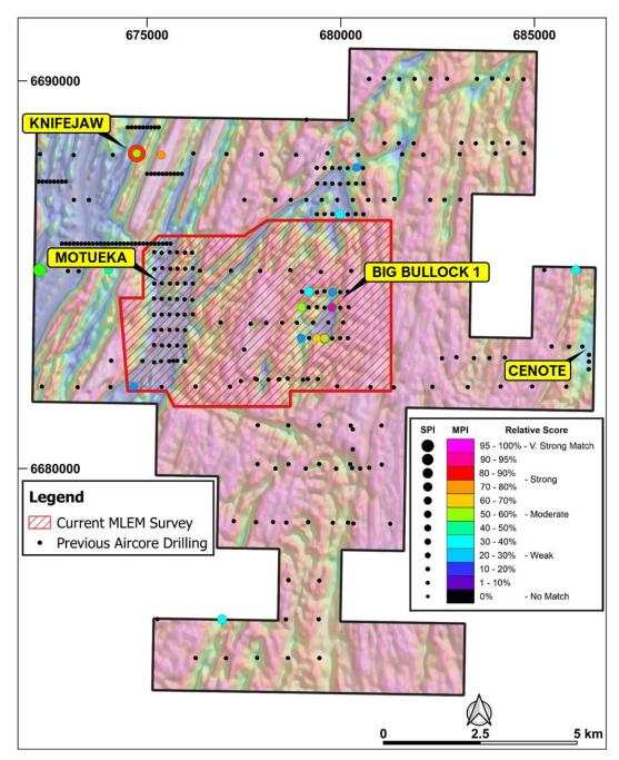
Figure 12: Big Bullocks tenement prospects with results of basement Prospectivity Index analysis and current MLEM survey outline (RTP magnetic image).
