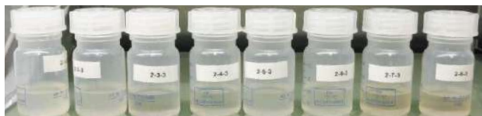
Figure 3. Electrolyte samples showing discolouration – Left to Right, 4N Alumina (99.99%), 3N Alumina (99.9%), Boehmite (99.7%)
