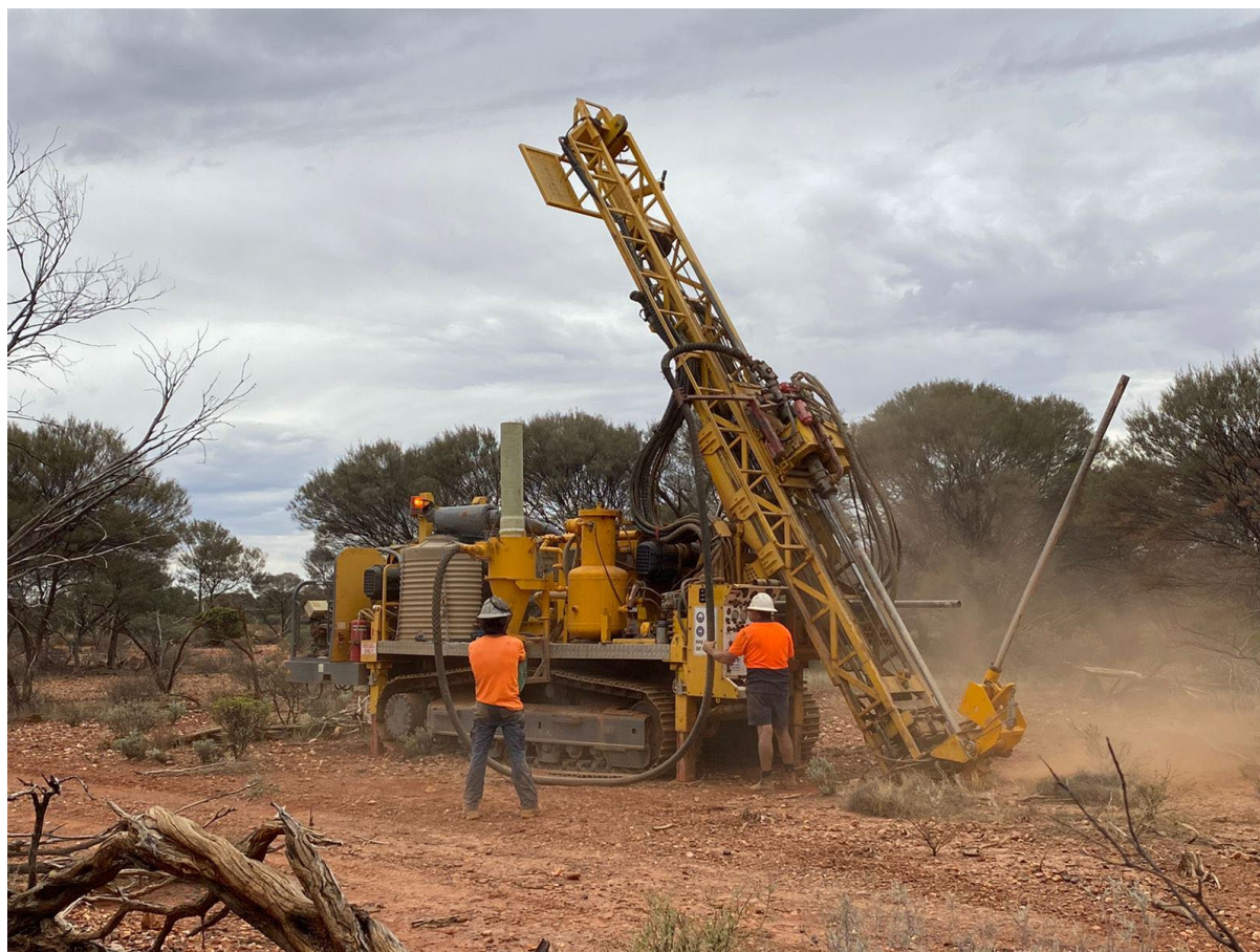
The RC drilling of the 800 metre Bulgera South gold anomaly was conducted by HARMEC Pty Ltd using this Edson 3000W track-mounted drill rig.
