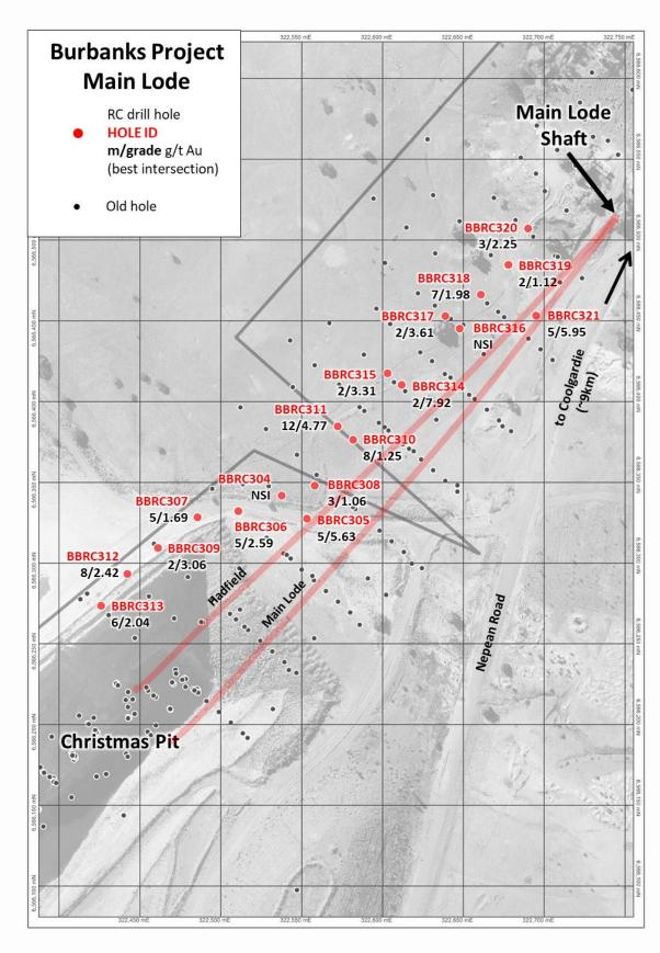
Figure 4 - Drilling Results at Main Lode
