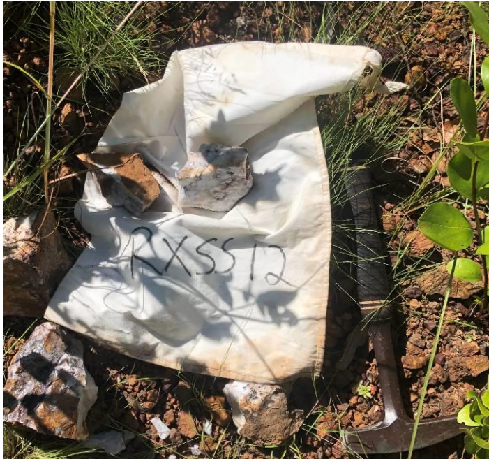
Plate 1 - RXSS12 – Quartz vein in ferruginous siltstone grading 3.8g/t Au
