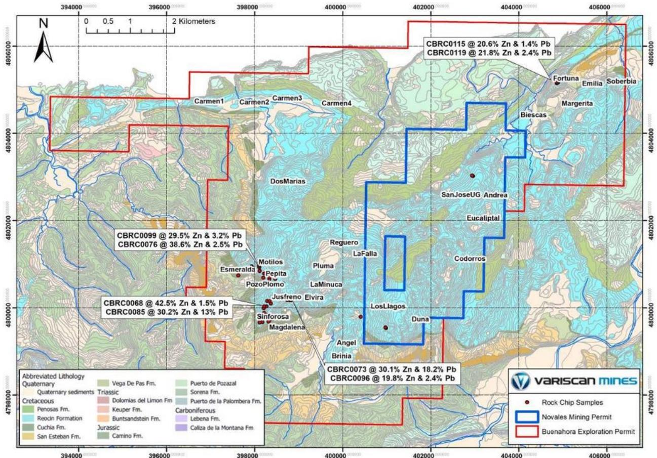
A work programme was designed for the Novales-Udias Project with the goal of establishing the presence of zinc mineralisation at surface and then defining the most prospective areas of mineralisation on which to plan a targeted future drill campaign. The work focused on progressing the exploration south-west of the Udias area across the Magdalena, Pozo Plomo-Jusfreno and Motilos-Pepita prospects.
