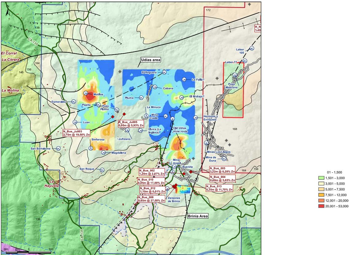
Note: Historic drill-holes which include intercepts grading over 2% Zn are indicated with red symbols. Historic drill holes that report intercepts under 2% Zn or are barren are indicated by grey symbols. Significant drillhole intercepts over distinct intervals are annotated.
