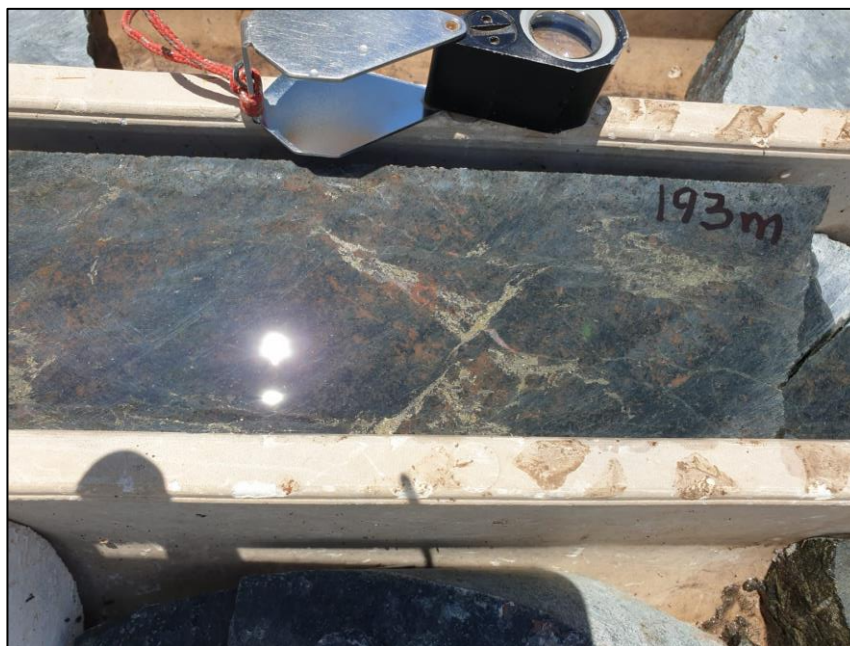
Figure 5 – drill core from DD hole KKODD004 showing gold-bearing pyrite-carbonate vein mineralisation through intensely altered mafic rocks within a high grade gold intercept (6m at 10.4g/t gold from 189 to 195m).
