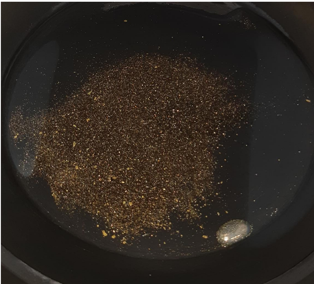
Figure 7: Gravity concentrate recovered from the Viago Lode 10 kg sample showing abundant gold grains.
