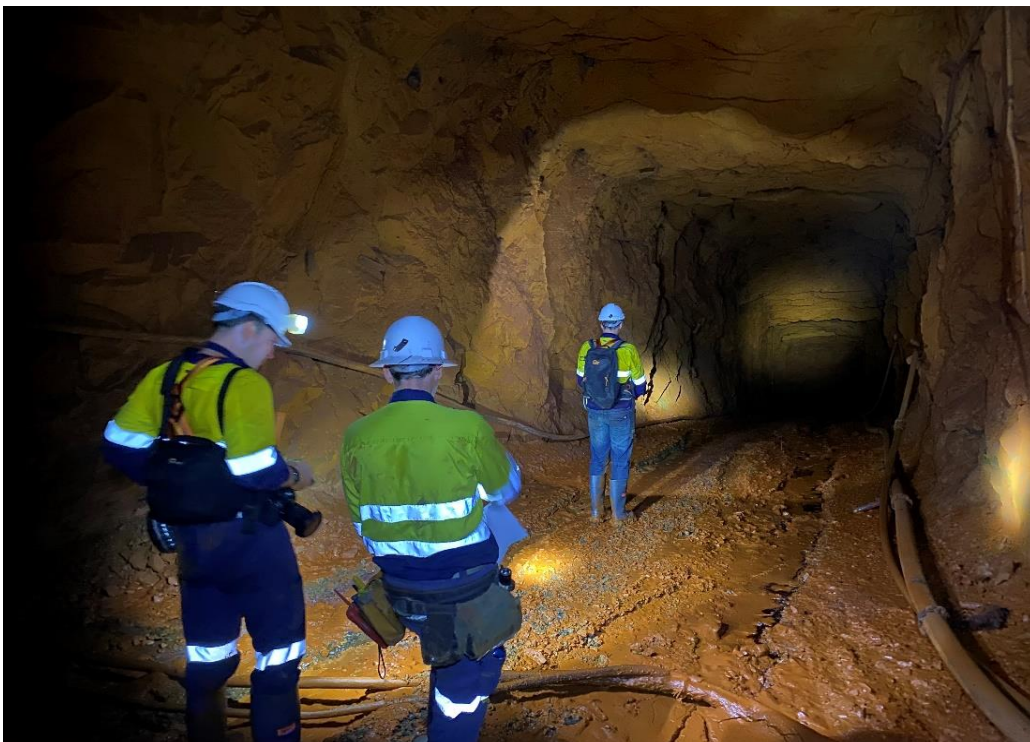
Figure 8: Bellevue technical staff inspecting the recently exposed main decline at the Bellevue underground mine during dewatering activities.
