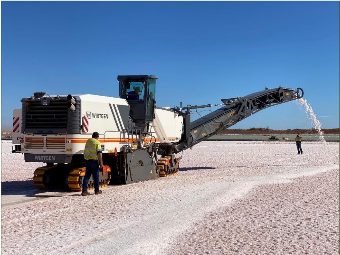
Wirtgen Salt Harvester Commissioning – June 2020
