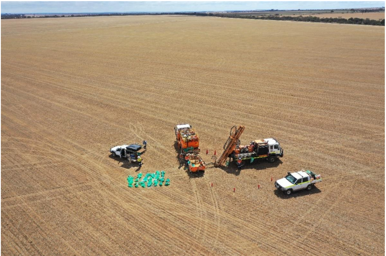
Figure 4: Air core drilling at Crossroads prospect March 2020 with 'Low Impact Rig', Burracoppin Gold Project
