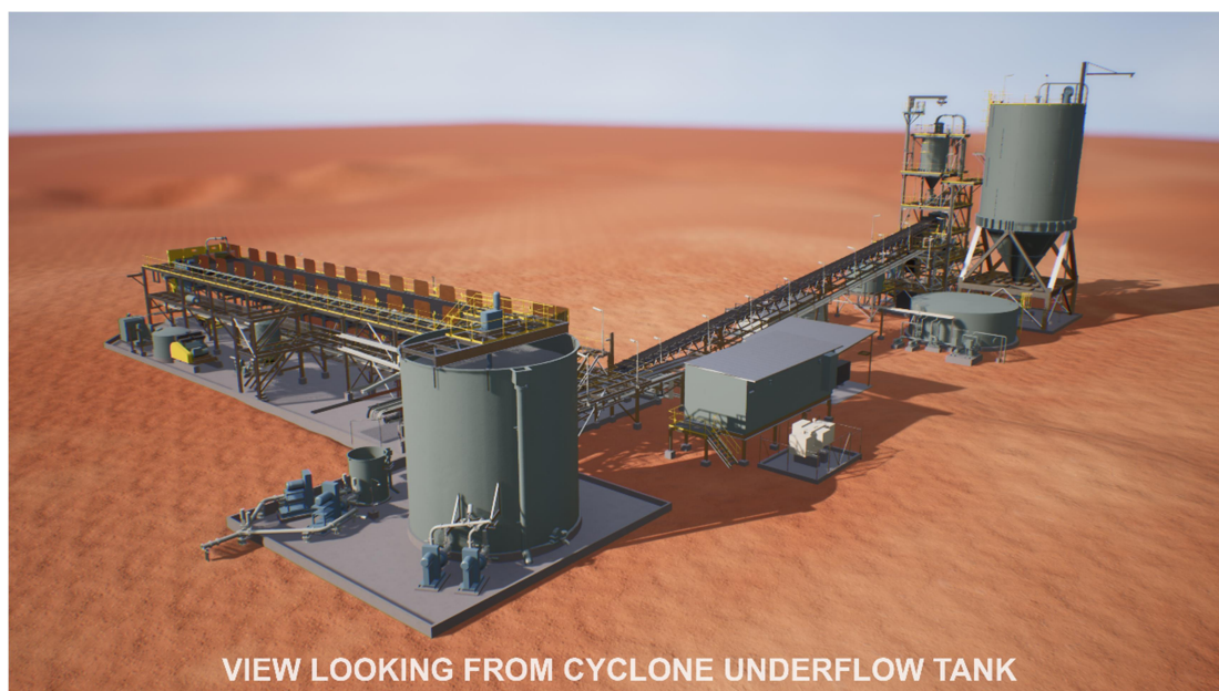
Figure 19 - Thunderbox paste backfill plant design
