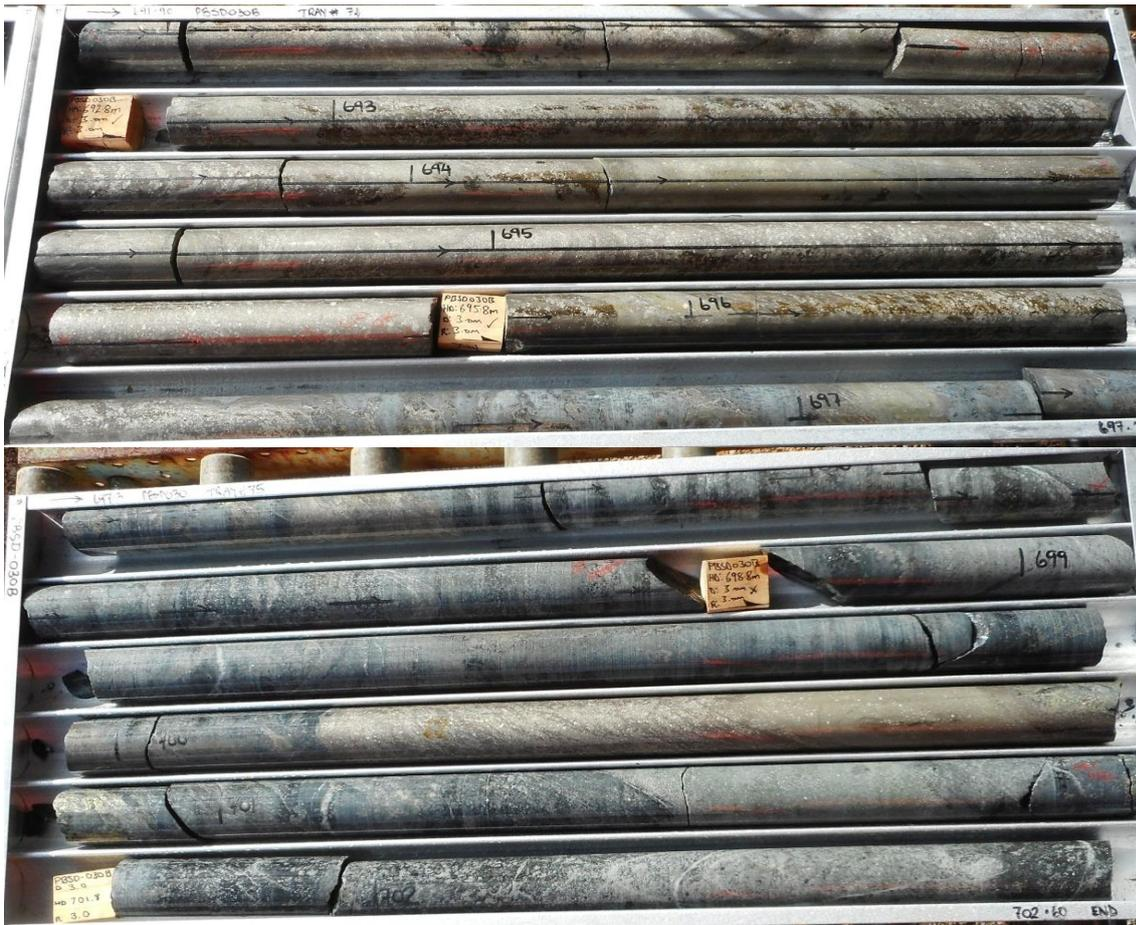
Figure 2 – Massive and stringer nickel sulphides in drill core from PBSD0030B
