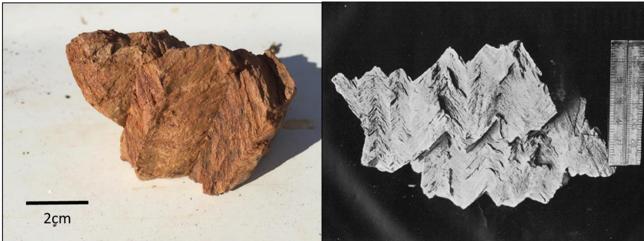
Figure 2: Left: Chevron folded sediments collected east of a series of substantial historic shafts at the Reward Prospect during recent mapping. Right: Chevron folds in sediments nearby to the high-grade gold lode from a cross-cut on No. 3 Level in the Mt Boppy Mine (Source: NSW Mineral Resources Publication No. 18 – 1913).
