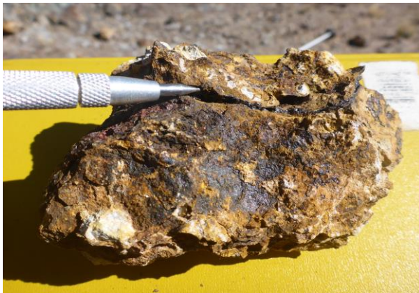
Figure 5 ABOVE LEFT: Sample from an epithermal vein at Colina Roja with 6.5g/t gold and 194g/t silver; ABOVE RIGHT: Sample from an epithermal vein at Uchpanga with 2.65/t gold and 920g/t silver.
