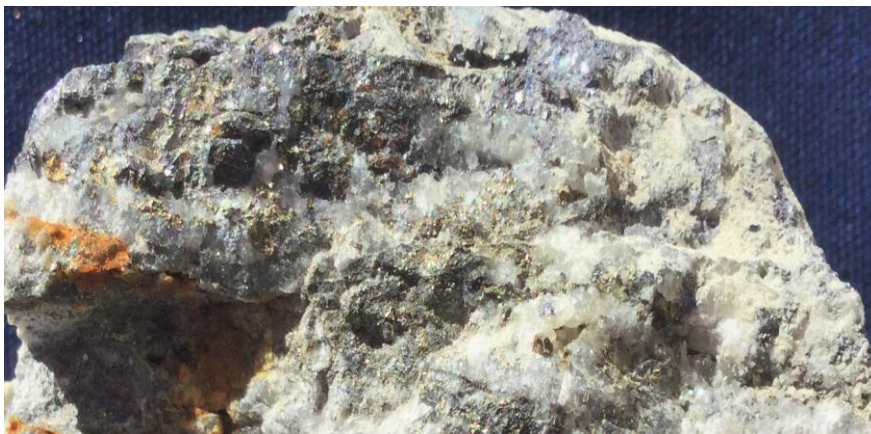
Figure 5 ABOVE LEFT: Sample from an epithermal vein at Colina Roja with 6.5g/t gold and 194g/t silver; ABOVE RIGHT: Sample from an epithermal vein at Uchpanga with 2.65/t gold and 920g/t silver.
