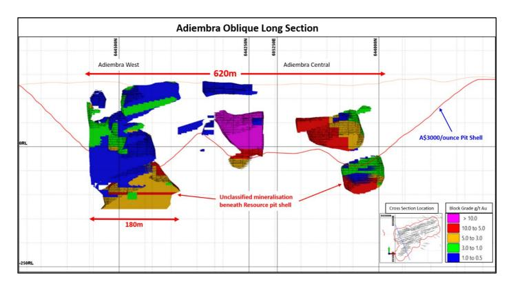
Figure 3: Adiembra Long Section showing plus 0.5 g/t blocks and Resource pit shell
