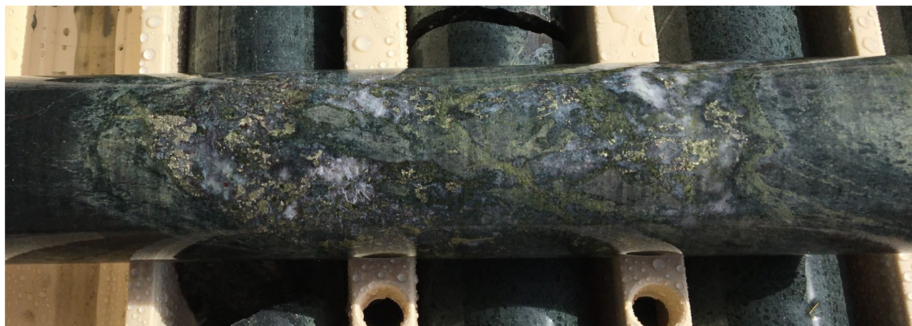
Figure 1. The best intersection of visual chalcopyrite (435.6m to 435.75m) part of the mineralised zone (423m to 438m). NQ core.
