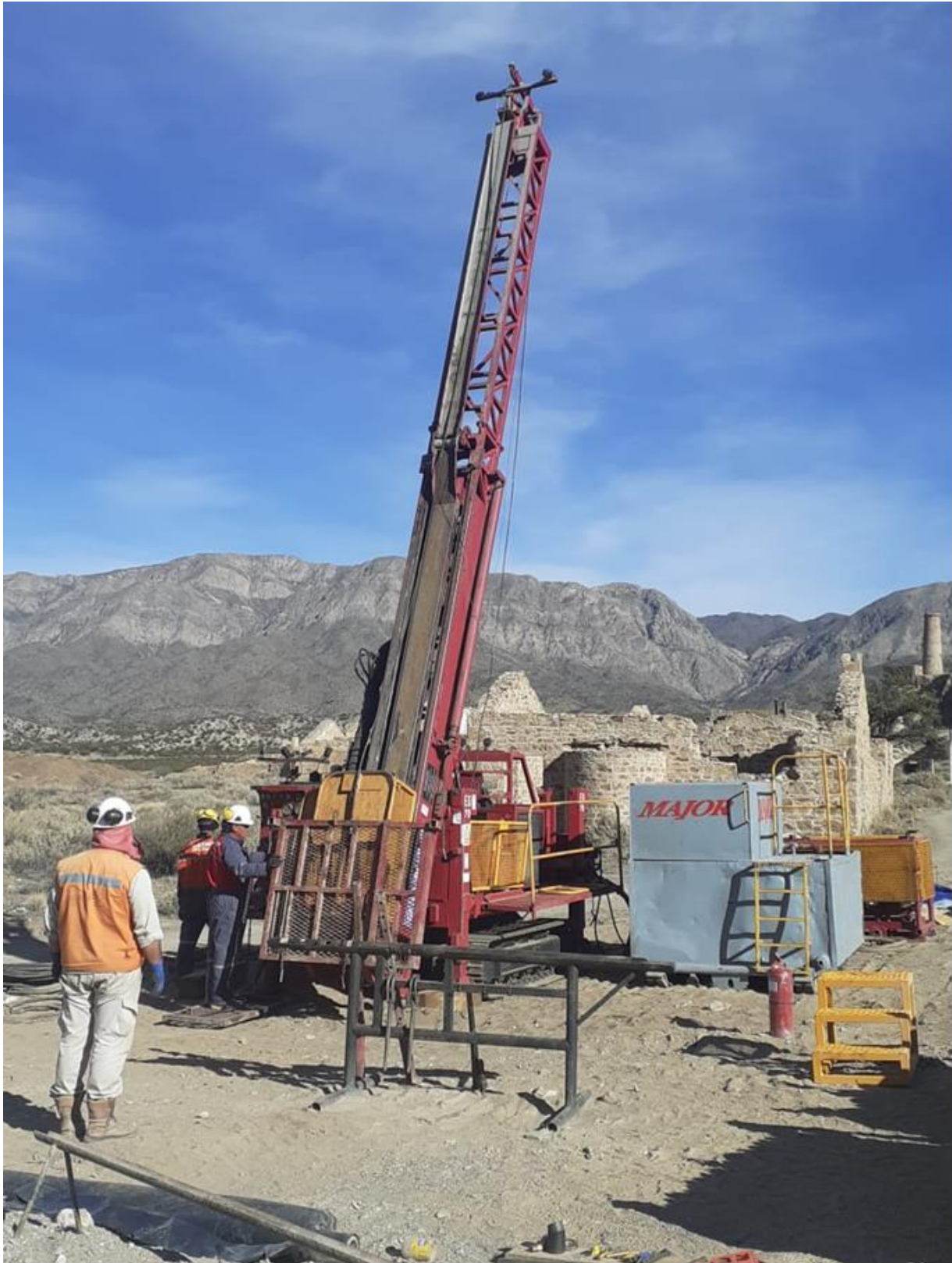
Photo - new Major Drilling diamond core rig on site and drilling hole GNDD-073 at Sentazon
