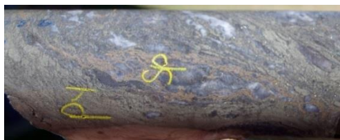
OFDD001 @ 246m: sheared massive pyrite & sphalerite
